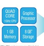
CPU, GPU, and memory are all included in an SoC (System on a Chip).
