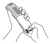
2 Insert the batteries negative (⊝) end first.
