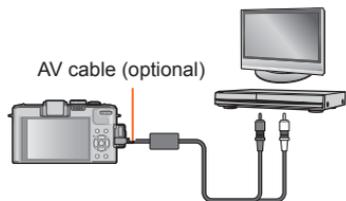
To recorder's input socket
